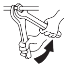
Two wrenches required to prevent damaging the copper piping.
